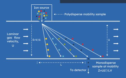
In the P5 parallel plate Differential Mobility Analyzer (DMA), sampled charged molecules or particles are simultaneously subjected to a gas flow and an electric field, such that only those with a specific mobility are transmitted into the DMA outlet.
