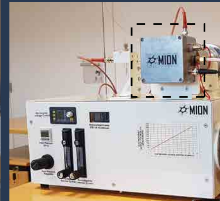
Figure 3: MION's aerosol electrometer coupled to a Half-mini DMA. The optimal amplification for the Half-mini DMA is 10^{12} V/A.
